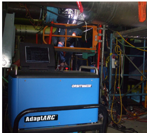
Above: Typical work area showing limited radial clearance for operation, making a light, modular system the perfect choice.
