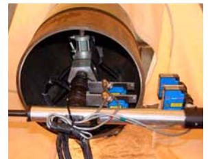
Laser Dimensioning System recording measurements for ID bore matching.
