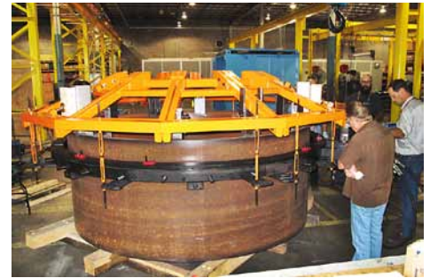
The new RBL is designed to operate with lifting/support frame.
