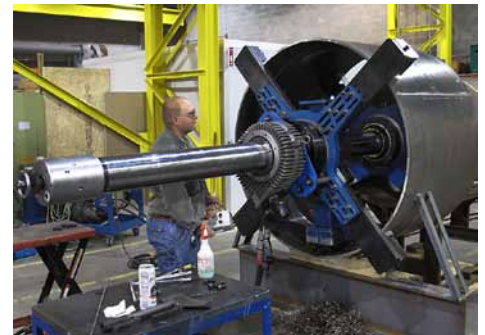
The classic Model 224B in a non-classic role as the primary weld prep tool for a special land-based pipeline with Inconel lined bore.
